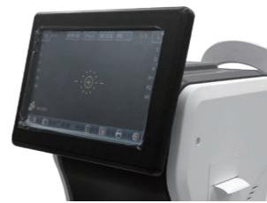
High brightness and contrast 9" wide color TFT LCD screen, smooth touch mode, different angle can be adjusted
